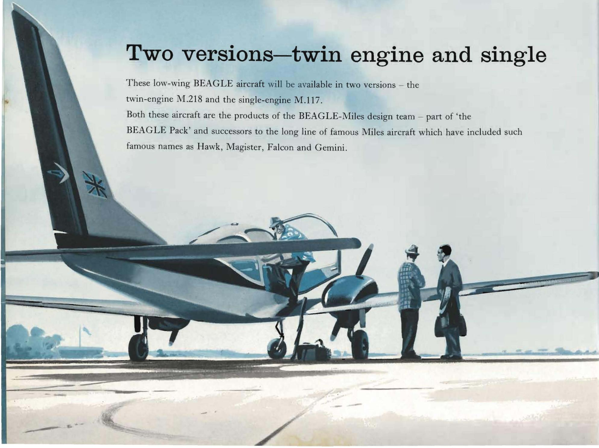
The BEAGLE M.218 is a light-twin four-seat high performance, low-wing monoplane. Although constructionally similar to its 'Kennel mate' the M.117, it has two 100 b.h.p. Rolls-Royce Continental O-200-A engines instead of one.
